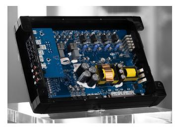
Easy Control Access – The amplifier was intentionally designed with sound controls located on the side panels, instead of the top panel, making it easier to access gain and crossover controls when installed under vehicle seats or in shallow-depth locations. Removable end caps were added to cover the side controls and connections, providing a clean, sleek finish to the amplifier.
